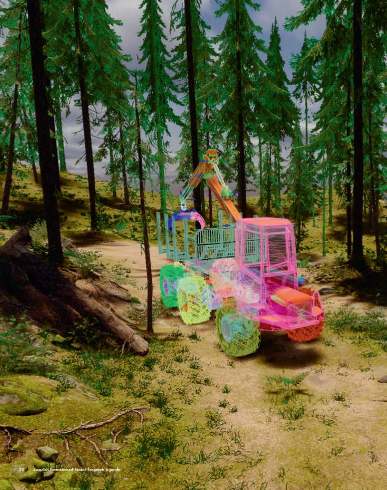
Simulation models are combined with forest data from laser scanning to develop autonomous functions, and to predict which routes are the easiest to navigate and the most environmentally friendly. Here we see a simulation model of the XT28 concept forwarder in a virtual forest.
